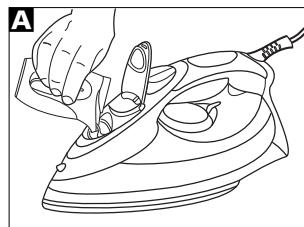
After filling, replace the fill cap.
